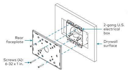
**NOTE:** Four washers are provided to secure the faceplate to the electrical box if the mounting holes are too large for the included screws.
