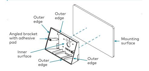
**CAUTION:** Allow a minimum of 24 hours for the adhesive to cure to the surface before installing the TSW-770/1070 Mounting Bracket. Failure to properly cure the bracket to the mounting surface could cause the MSMK to detach after installation.
